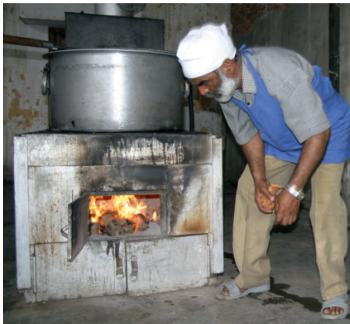
Nishant Bioenergy's cookstove – using crop waste instead of LPG
